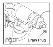
To drain the pump, remove the access panel from the spa unit (see ATTACHING AND REMOVING THE ACCESS PANEL on page 14). Locate the pump inside the spa unit. Remove the drain plug from the pump and allow all water to drain from the pump. Replace the drain plug.
